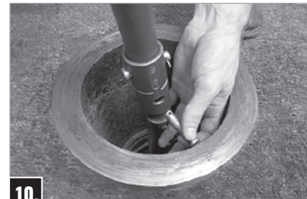
10. Remove the Upper Valve Rod and Traffic Rod Coupling as a unit by removing the lower Cotter Pin and lower Clevis.
