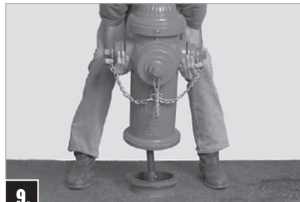
9. Remove Standpipe Traffic Coupling and lift Upper Standpipe and Bonnet assembly straight up and off of Valve Rod. DO NOT lose Standpipe Coupling Seal.
