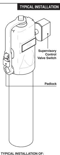
TYPICAL INSTALLATION OF: U-20806: 4" - 14" Post Indicator Valves U-20807: 16" - 24" Post Indicator Valves
