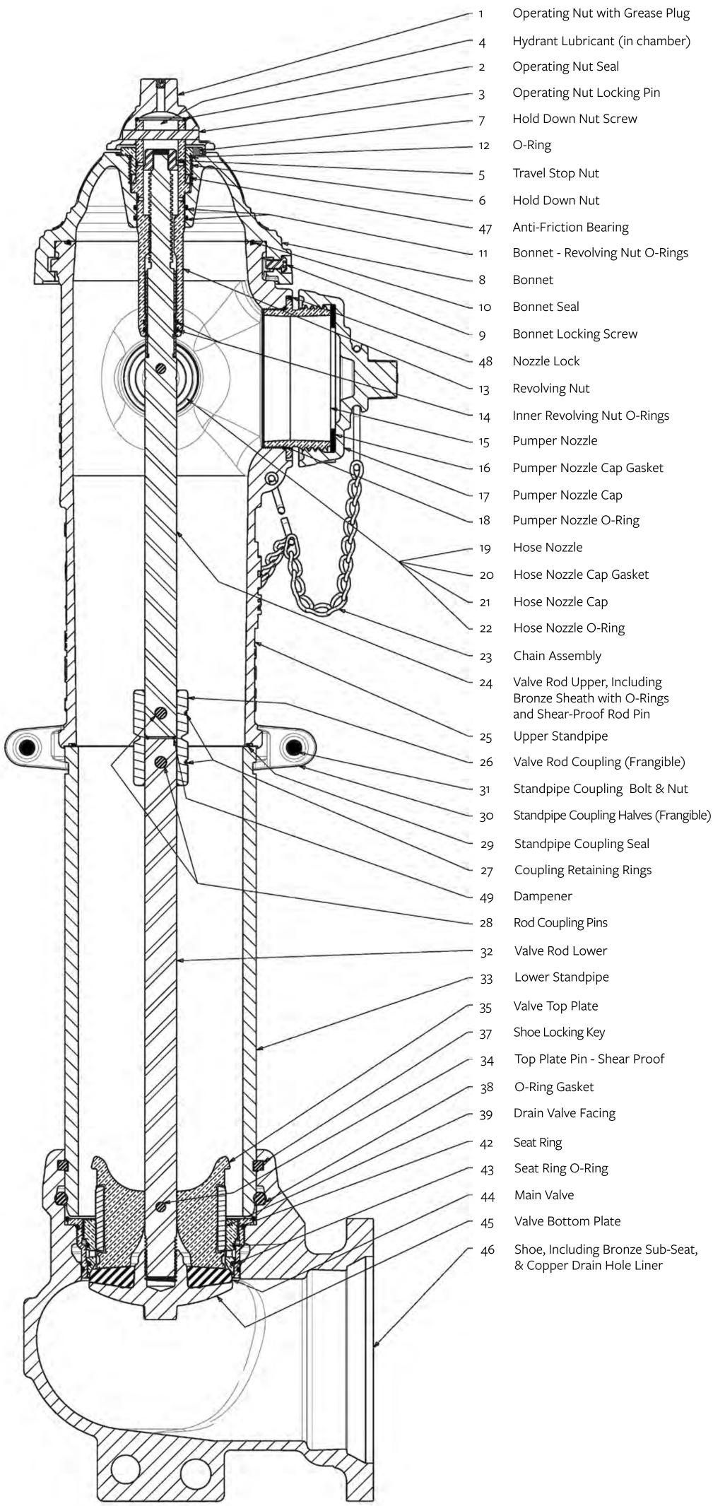
Operating Nut with Grease Plug Hydrant Lubricant (in chamber) Operating Nut Locking Pin Hold Down Nut Screw Anti-Friction Bearing Bonnet - Revolving Nut O-Rings
