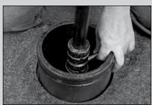
2 Slide bottom Coupling Retaining Ring out of groove, remove bottom Rod Coupling Pin and separate Upper Valve Rod with Valve Rod Coupling still attached from Lower Valve Rod. Remove and save Dampener ring.
