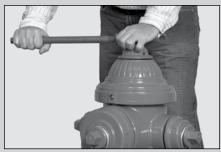
**5** Close the hydrant Main Valve first, then open the auxiliary hydrant control valve. Operate the hydrant and check for leaks.
