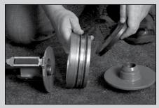
4 Remove and inspect rubber Main Valve. Remove bronze Seat Ring by sliding down off guides of Valve Top Plate – inspect and replace, if damaged. Replace Seat Ring O-Rings, if damaged.
