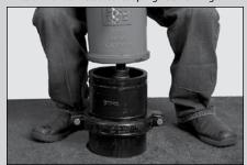
Place Upper Standpipe on Extension, taking care to keep Standpipe Coupling Seal in place during assembly.
