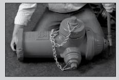
3 Clean all mating parts as needed. Turn Operating Nut to fully "open" position, so bottom of Upper Valve Rod slides out as far as possible.
