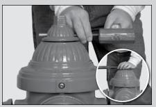
Tipove out Operating Nut Locking Pin from rounded side of Operating Nut. Remove Operating Nut, while taking care not to lose Operating Nut Seal, which is located inside the Operating Nut. With an 1/8" Allen wrench, loosen Hold Down Nut Screw – then remove Hold Down Nut using the Combination Spanner Wrench by turning counterclockwise.
