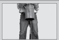
■ Depth of bury for this hydrant can be extended in 6" increments by using a standard Extension Kit, available from 6" to 36" in length. Longer lengths are special order. Follow steps 1 & 2 for bonnet removal on Page 7. Then, remove frangible Standpipe Coupling and lift Upper Standpipe over Valve Rod, taking care not to lose Coupling Seal in the process.
