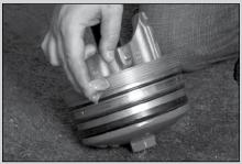
Lay out all components, replacing worn, damaged ones as needed. Clean first, then grease all threaded parts, using a lubricant such as Diana 2100 (replacement grease must be compatible with calcium sulfonate grease). After lubrication, reassemble parts and securely tighten Bottom Valve Plate.
