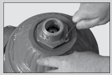
Re-grease both upper and lower chambers of Revolving Nut. Then, reinstall Hold Down Nut and tighten securely. Install and tighten Hold Down Nut Screw, and finally reinstall Operating Nut and Operating Nut Locking Pin.
