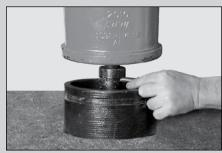
Set the Upper Standpipe with the Upper Valve Rod extended down over the Lower Standpipe. Guide the bottom of the Upper Valve Rod into the Valve Rod Coupling, line up holes and install Pin – there is space enough to do this. Slide the second Coupling Retaining Ring down so it snaps back into its groove, locking the Pin in place.
