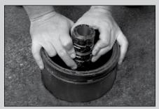
Install new Valve Rod Coupling, and slip stainless steel Coupling Retaining Rings up and out of grooves, for Pin removal. Put replacement Valve Rod Coupling over top of Lower Valve Rod—make sure Dampener ring is in place inside coupling at top of Lower Valve Rod. Replace lower Pin and slip Coupling Retaining Ring down, snapping back into groove and locking Pin in place.
